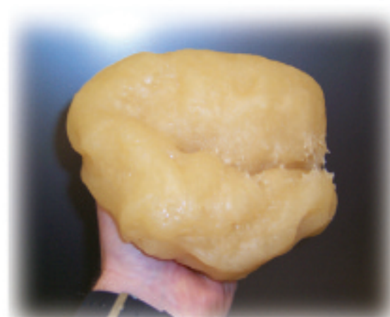
1/2 gallon of gasoline encapsulated using 150 grams of OXP-151
